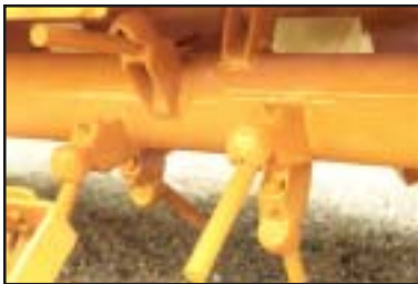
Northwest blades ( above ) are attached to adjustable rotors and break up soil better than spikes ( below ) or tines
