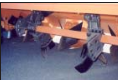
Northwest blades ( above ) are attached to adjustable rotors and break up soil better than spikes ( below ) or tines
