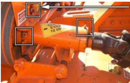
Grease will appear here when back bearing is filled full.
